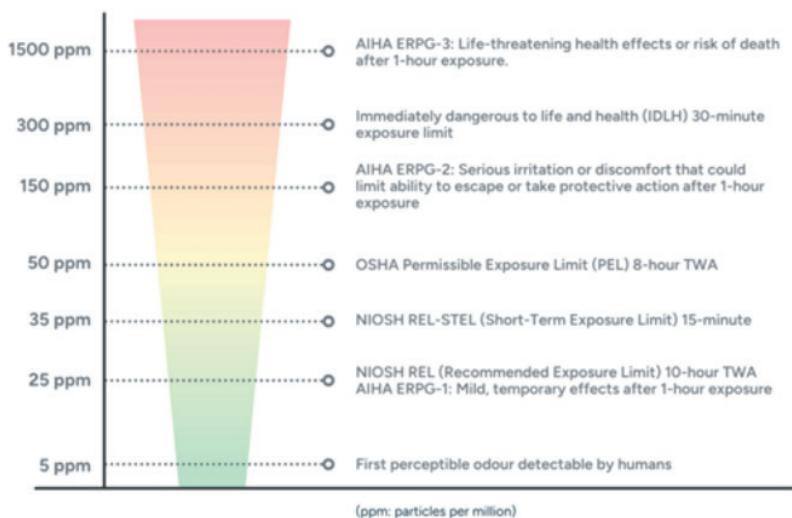
Overall, ammonia is both a valuable resource and a hazardous chemical. Safe handling requires understanding that as a liquid that boils at  $-33^{\circ}\text{C}$ , a leak can instantly create a freezing, choking cloud, and that emergency measures must be in place to protect anyone in the vicinity.
